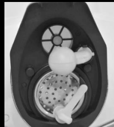
Fit the mask sensing tube to the fit test port (on a TSI PortaCount it is the clear tube).
